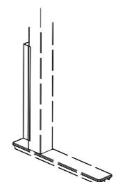
**passacavi verticale**, vertical cable carrier duct, chemin de câbles vertical, kabeldurchlass vertikaler, kabeldoorgangdop, pasacables vertical
