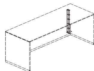
**passacavi verticale**, vertical cable carrier duct, chemin de câbles vertical, kabeldurchlass vertikaler, kabeldoorgangdop, pasacables vertical
